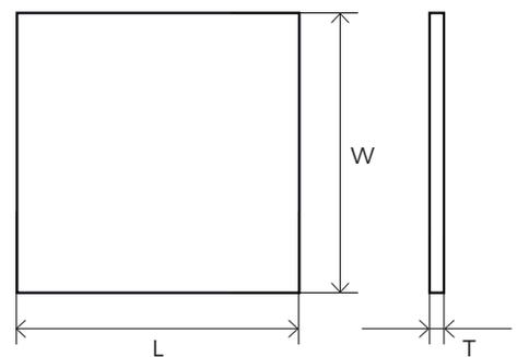
(a) For sizes with width and length equal to 105 mm, actual size can vary from 103.8 to 106.8 mm depending on grade selection. Tolerances on width and length are +1.5 / 0 mm.
